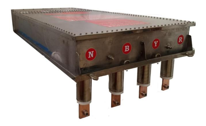
The HEMP power line filter design has been carried out for protection of utility 440 V, 3-Phase, 50 Hz power line. The HEMP power line filter is a combination of linear and nonlinear elements, which are used to mitigate the coupling effects of HEMP. The MIL-STD-188-125-1 lays down the detailed guideline for HEMP filter testing and qualifications.
