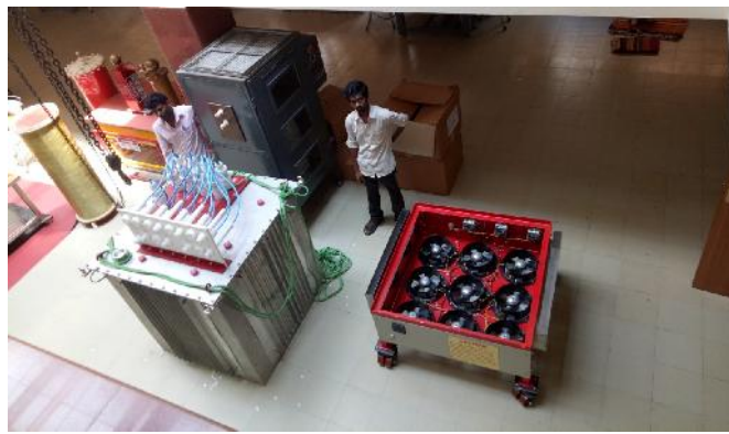
High Power Load Bank 150 Kilo watts /200 kilo watts
