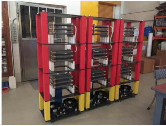
Very High Voltage Floating Load Bank Resistance + Inductive as loads
